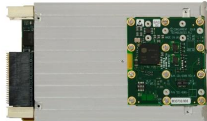
Figure 2: With M.2 Carrier and without 2LM Type 1 Covers
